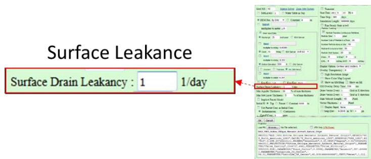
Figure 3-7: Surface leakance parameter text box.
