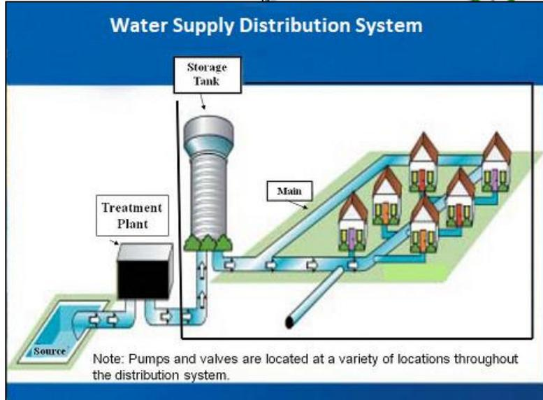
The diagram, titled 'Water Supply Distribution System', illustrates the components of a water supply network. It shows a 'Source' (lake) connected to a 'Treatment Plant', which feeds into a 'Storage Tank'. From the storage tank, water flows through a 'Main' pipe to a residential area with several houses. A note at the bottom states: 'Note: Pumps and valves are located at a variety of locations throughout the distribution system.'
