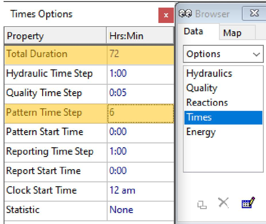
The screenshot displays two overlapping windows from a software application. The 'Times Options' window is a table with the following data:
