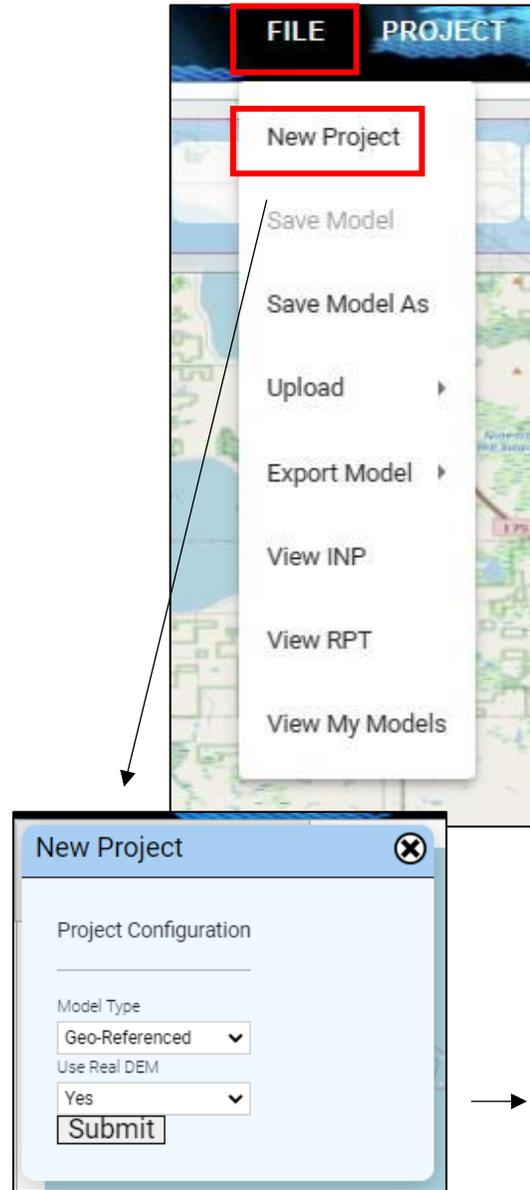
[Use this menu to start a new project, save the model file, upload an existing model, export the model map or model Geojson file, or view the model INP (input) file or simulation RPT (report) file.]
